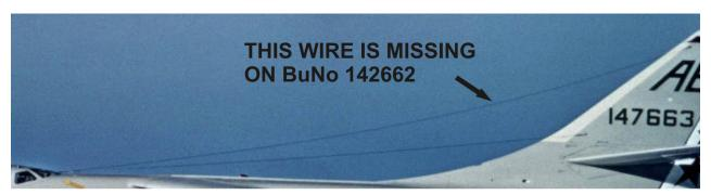
3. It seems every Skywarrior that had AN/ARN-59 DF system had it's antenna in its own shape and size. Antenna was located on the right side of the cockpit, and we provide you with design correct for BuNo 142662. Decal antenna comes in two identical pairs, each pair consists of two mirrored designs. Actually antenna was inside, on the inner surface of the canopy glass, so
